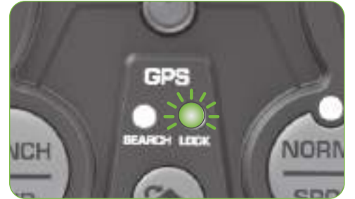
Once GREEN LOCK LED turns on solid, the drone is ready to fly.
