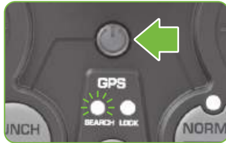
Turn on controller. Once paired with the drone, RED SEARCH LED will blink while acquiring GPS signal.
