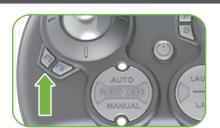
IF THE DRONE SPINS COUNTER-CLOCK-WISE (VIEWED FROM ABOVE): Press the 🔼 button several times until the drone stops
